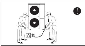
Make sure the power supply to the heat pump unit is off before any operations are done on the unit.
