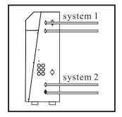
1) Connect one side of refrigerant pipe to the indoor unit (for both system 1 and 2).
