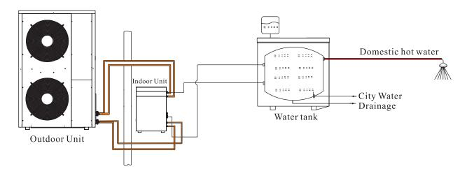
Application 2: The unit only supplys the hot water for floor heating. This installation is for supplying floor heating hot water only.
