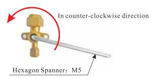
6) Take off the copper nut of the gas and liquid valves, open the valves with hexagon spanner as much as possible.
