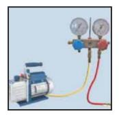
3) Prepare a vacuum pump and a pressure gauge, connect one tube of the pressure gauge to the vacuum pump.
