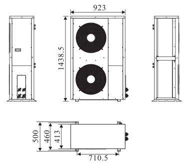
Liquid pipe O.D.  $\phi$  9.52 Gas pipe O.D.  $\phi$  12.7
