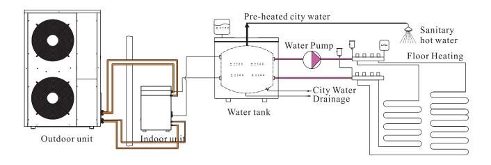
Application 4: This application integrated with solar panel can provide hot water for domestic use, floor heating and radiator (this application needs special multi-functional water tank). It provides hot water for central house heating and hot water system.
