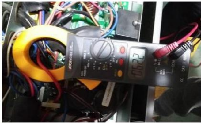
The current is 6.22A in the picture. If failure code F3 occurs, and the measured current is over than 1A, replace the outdoor PCB.
