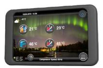
**User-friendly touch screen interface** The interface enables quick adjustment of all temperature settings directly from the front page. The software also supports variable temperature settings (curve) for both heating and cooling.
