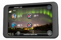
User-friendly touch screen interface The interface enables guick adjustment of all temperature settings directly from the front page. The software also supports variable temperature settings (curve) for both heating and cooling.
