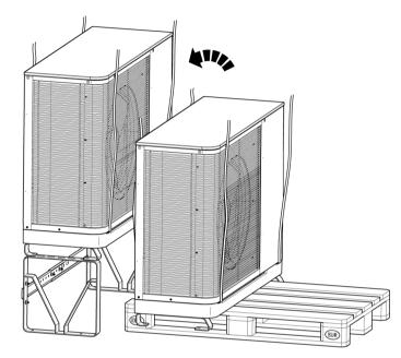
4 Use four bolts together with washer and nuts to attach the outdoor unit to the outdoor stand.
