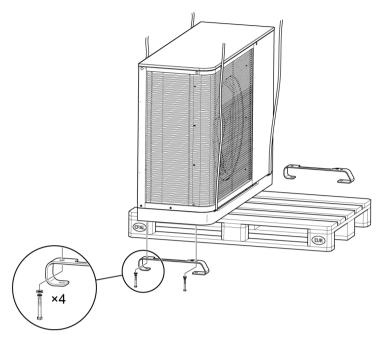
If the screws are difficult to attach, then adjust the outdoor unit's position on the drain pan.
