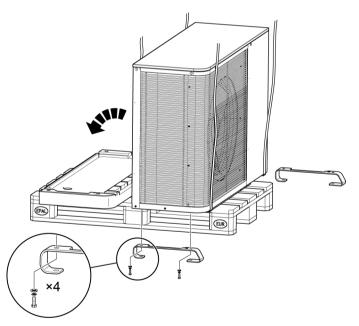
**5** Assemble the two feet with the longer bolts (M8  $\times$  100), spring washers and plain washers. Make sure to tighten the bolts.
