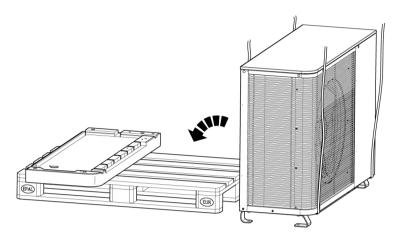
4 Remove the feet by unscrewing the four bolts, then lift the outdoor unit with the lifting straps. Place it on top of the drain pan.
