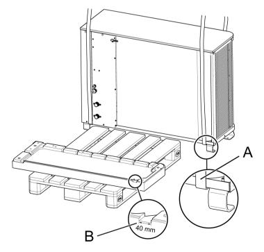
The drain pan has a slot (B = 40 mm) that will fit a 35 mm wide lifting strap, once the outdoor unit is placed on it.
