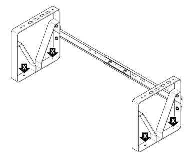
2 Choose proper fixations and attach the stand to the foundation, in order to avoid tipping of the outdoor unit.
