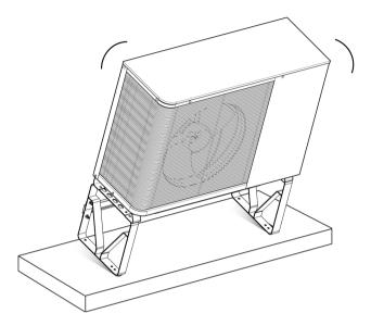
**3** Lift the outdoor unit and place it on top of the outdoor stand, using appropriate lifting equipment.
