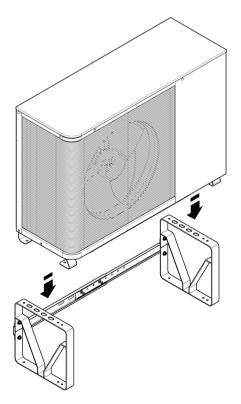
4 Use four bolts together with washer and nuts to attach the outdoor unit to the outdoor stand.
