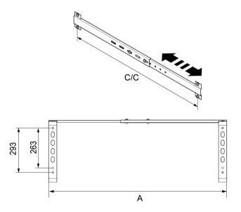
Tightening torque for the bolts is 22 Nm.
