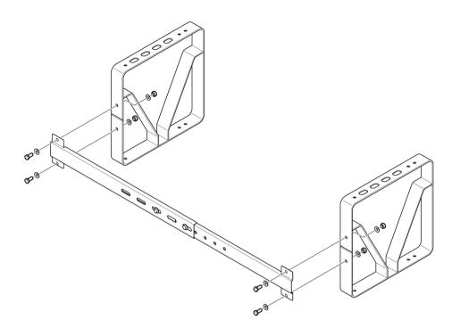
Tightening torque for the bolts is 22 Nm.
