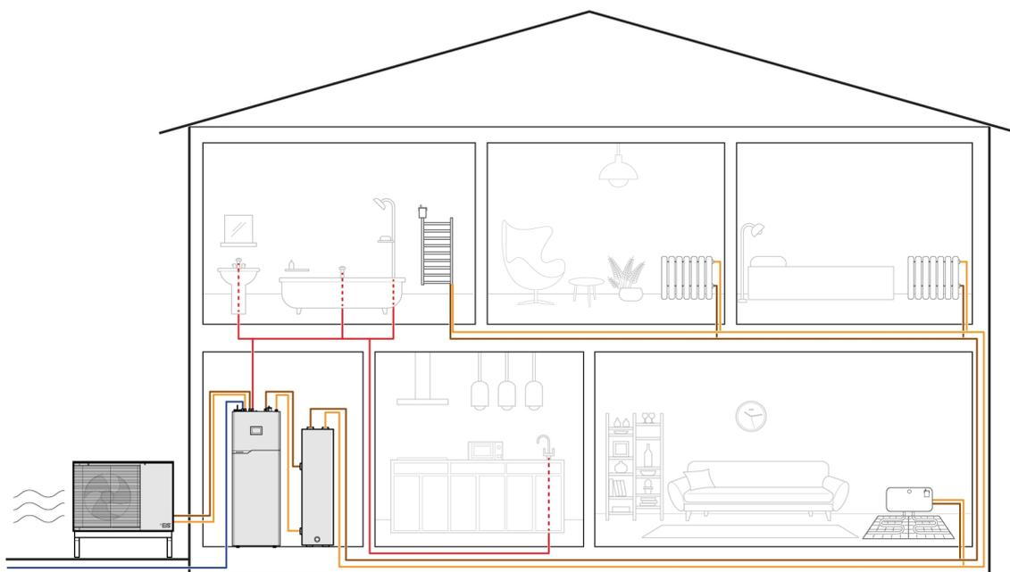
An air-to-water heat pump takes advantage of the energy in the outdoor air, using it to heat water for use in the household and for different types of space heating.
