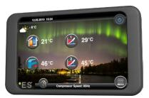
User-friendly touch screen interface The interface enables guick adjustment of all temperature settings directly from the front page. The software also supports variable temperature settings (curve) for both heating and cooling.
